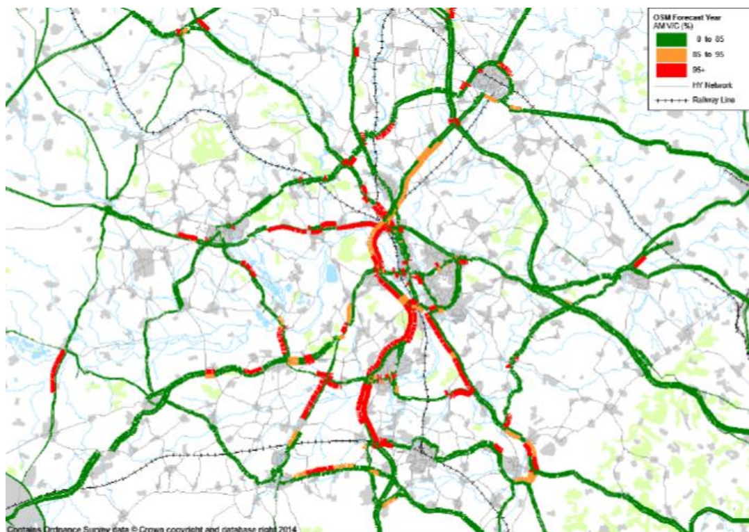
Figure 15: Highway Network in the morning peak in 2031 with no intervention – volume of traffic in relation to road capacity (85% to 95% = at capacity, 95% plus = over capacity)
